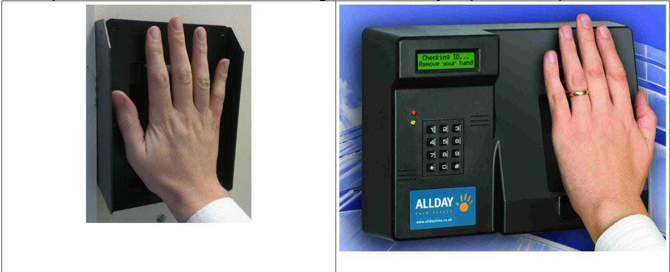
If the reading is successful, your staff number and possibly your name will appear on the LCD screen. If you are using an external separate reader unit you should see a green LED light up on the reader casing indicating the read was successful. Also the terminal will release the door for a few seconds so that you can gain entry.
